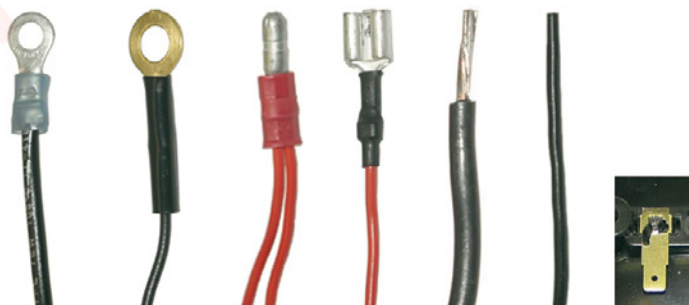
All non-insulated connections, clipped, stripped or tinned ends
